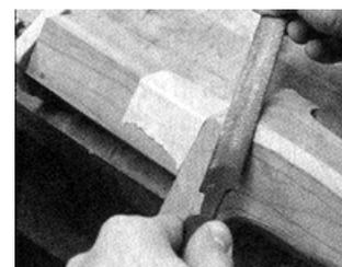
**Fig. 4** Shield the corner from damage with tape.
